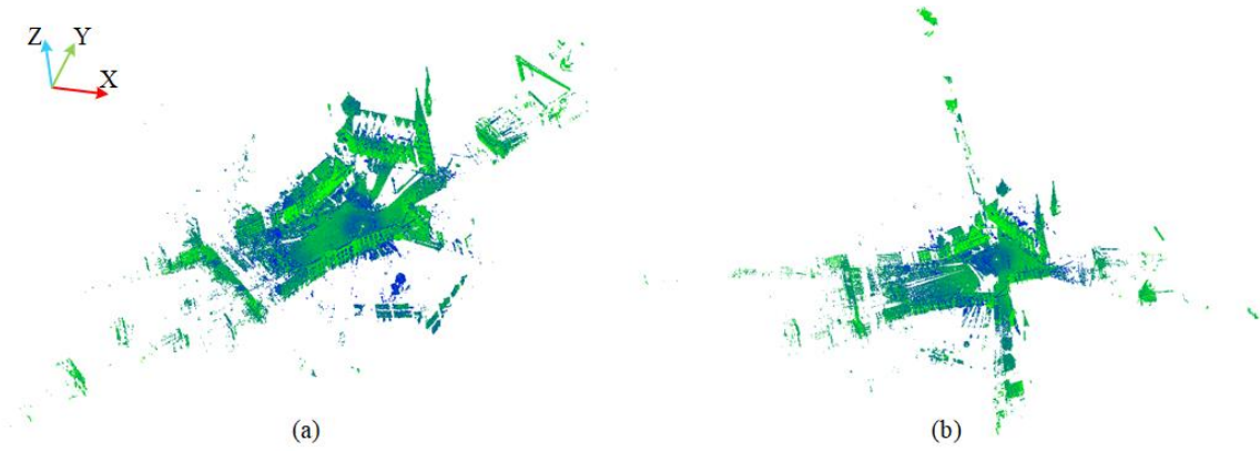
Figure 6.1: The Bremen TLS dataset. a) Target and b) source point clouds color-coded with intensities.
