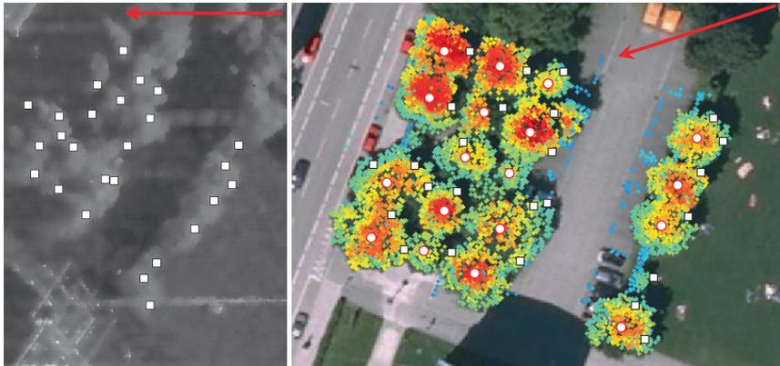
Fig. 5: Local maxima (white boxes) detected in the SAR intensity image (left). These maxima are projected into an orthophoto (July 2009) overlaid with a LiDAR point cloud (September 2009) in order to show their real world position (right). The SAR viewing direction is indicated by the red arrows. The red circles indicate manually determined tree top positions. Note how all detected maxima are located towards the sensor.
