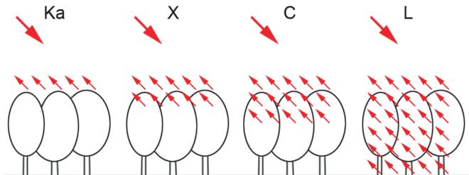
Fig. 1: Tree canopy penetration of common SAR wavelengths.
