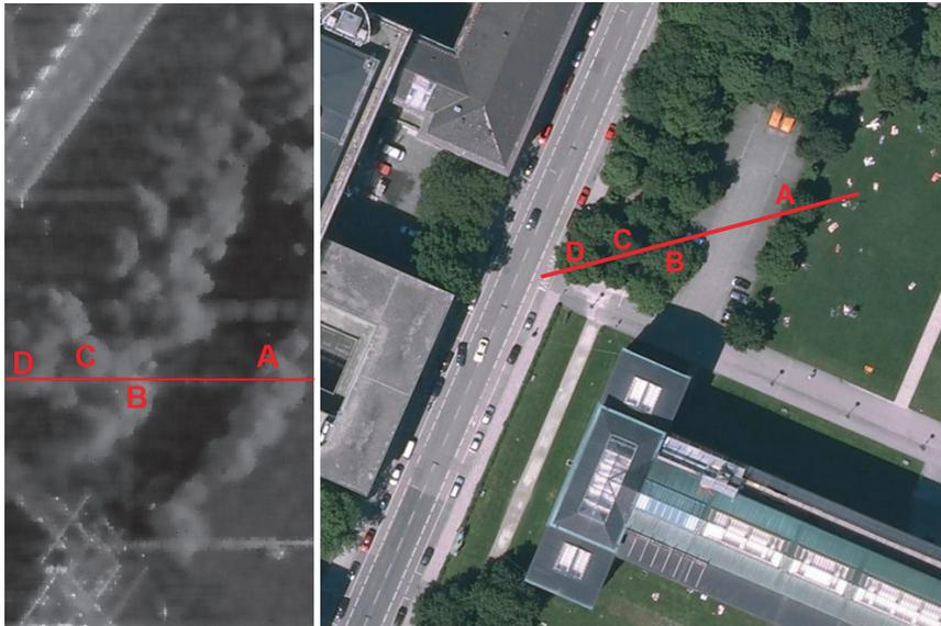
Fig. 2: SAR intensity image in slant range geometry (left), orthophoto of the "Alte Pinakothek" test scene (right). The red line indicates a range profile corresponding to the radar's viewing direction. A, B, C and D are trees appearing in this range line.
