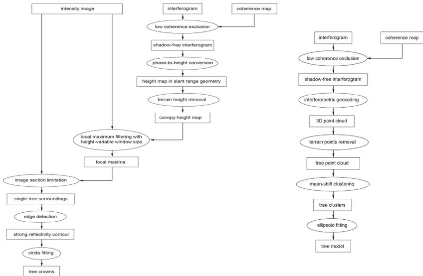
Fig.6: Workflows of the proposed tree recognition concepts. Left: Image-based approach. Right: 3D-based approach.
