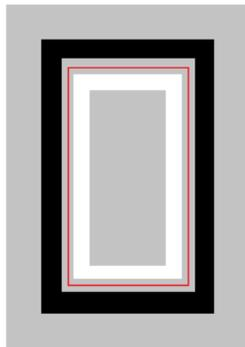
Figure 3. Mask used for correlation: red – expected shape of the window; black & white – binary mask; grey – don’t-care-areas
