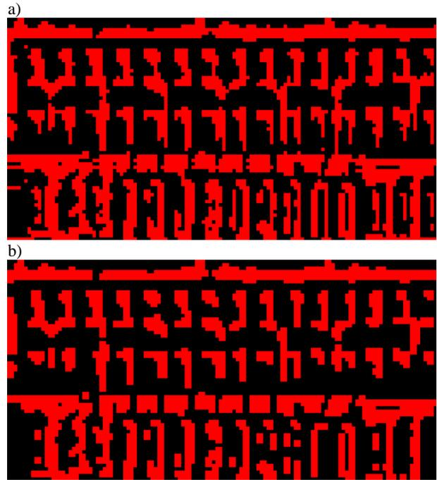
Figure 4. a) Extraction of candidates for windows from IR texture using local dynamic threshold; b) separation of the regions and removing false detections using morphological operations
