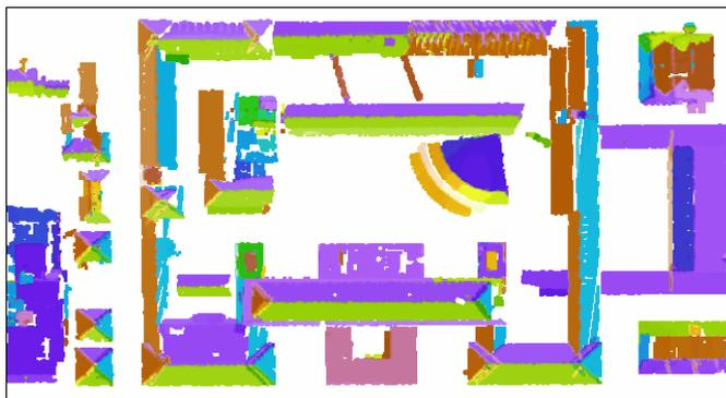
Fig. 2. Top view of the point cloud after removing clutter objects. Color coded map according to the estimated normal <sup>[10]</sup>.
