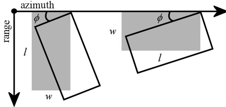
Figure 3.3: Definition of width  $w$ , length  $l$ , and aspect angle  $\phi$  of a building. The buildings in gray are oriented parallel to the azimuth direction with  $\phi = 0^\circ$ , while the buildings with the solid black lines were rotated by  $\phi$  with respect to the azimuth direction.
