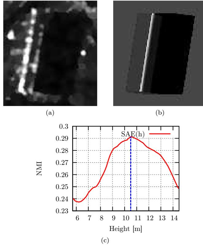
Figure 7.10: RMA example for the undamaged building shown in Figure 3.5 using  $SAE$  (7.3) as the similarity measure. (a) Image subset of building in filtered post-TSX scene. Simulation and actual scene are coregistered. (b) Simulated building at height where the similarity is highest ( $h = 10.5$  m). (c) Plot of similarity as a function of height. (SAR image: Infoterra GmbH/DLR, 2008.)
