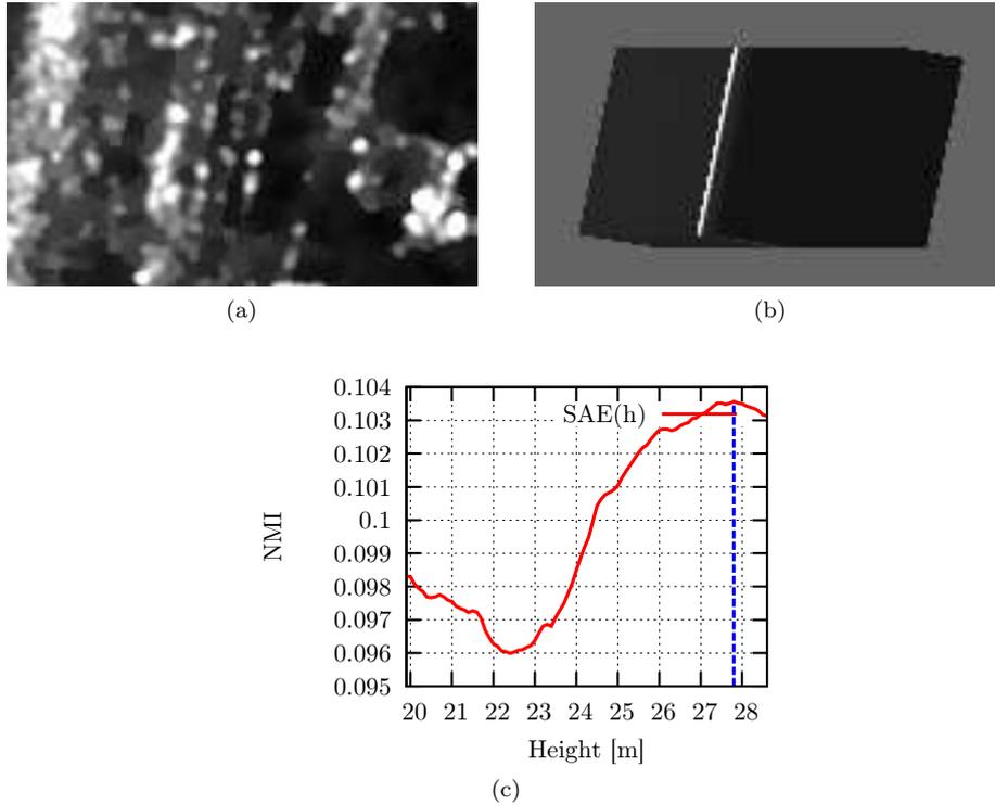
Figure 7.11: RMA example for the damaged building shown in Figure 7.3 using  $SAE$  (7.3) as the similarity measure. Viewing direction is from the left. (a) Image subset of building in filtered post-TSX scene. (b) Simulated building at height where the similarity is highest ( $h = 27.8$  m). (c) Plot of similarity as a function of height. (SAR image: Infoterra GmbH/DLR, 2008.)
