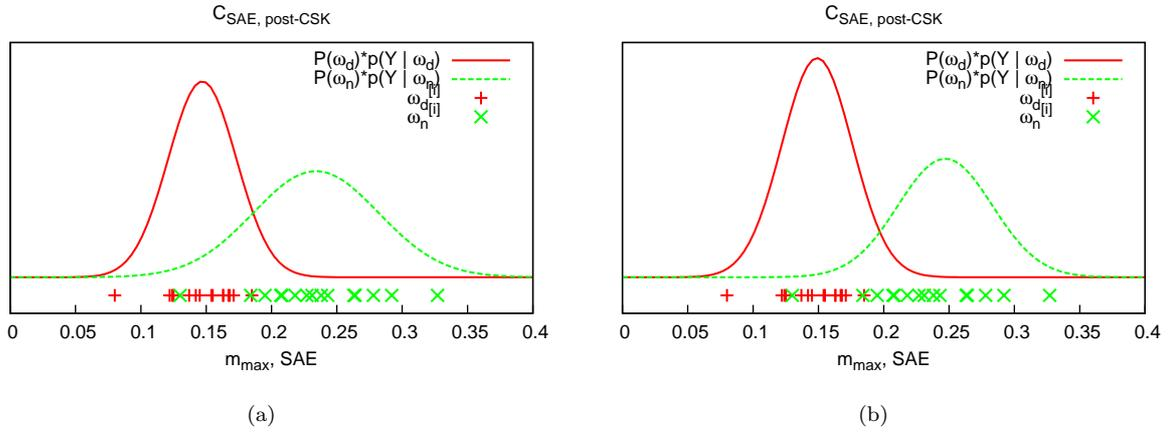
Figure 7.13: Comparison between supervised and unsupervised  $C_{SAE,post-CSK}$  classifiers. In this example the EM algorithm estimated the parameters for the unsupervised classifier with a good accuracy. The symbols “+” and “x” denote the actual  $m_{max}$  values of the buildings in class  $\omega_d$  and  $\omega_u$ , respectively. (a) Supervised classifier. (b) Unsupervised classifier.
