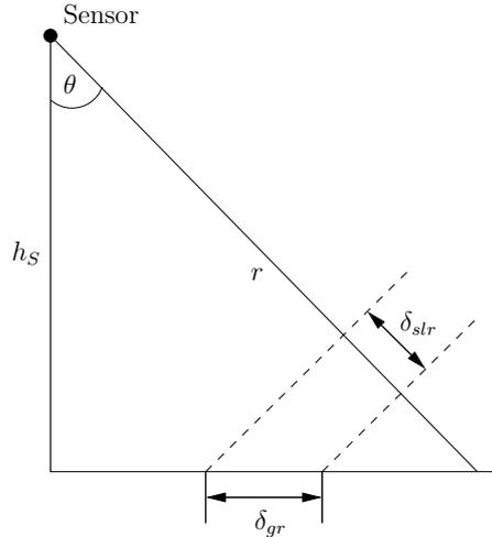
Figure 2.4: Geometry in slant- and ground range projection.
