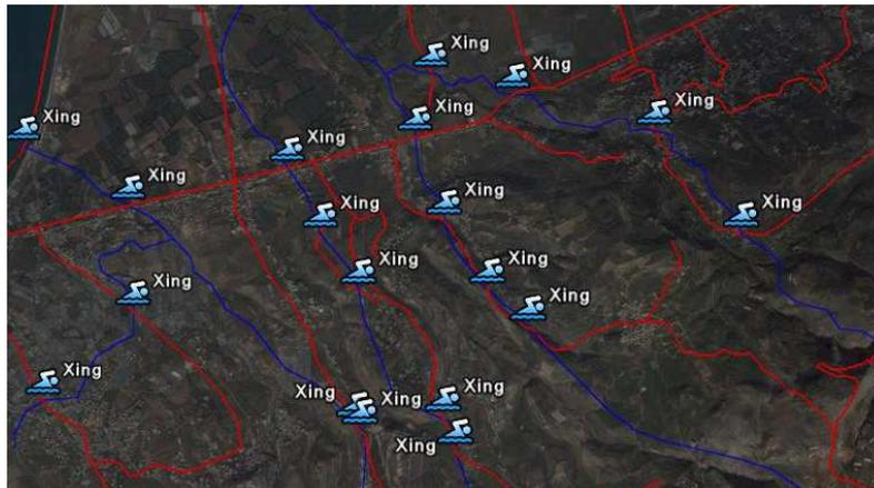
Figure 8.8: An example of automatic derived road-water crossings. The geospatial intersection function was applied to the road (red) and river (blue) networks resulting in the highlighted crossings. (Satellite image: Space Imaging International Ltd. distributed by European Space Imaging GmbH, 2005.)
