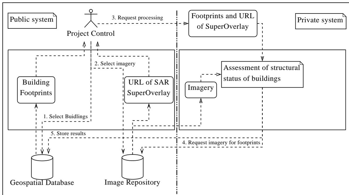
Figure 8.6: A schematic overview of the integration of the damage assessment method into the system.
