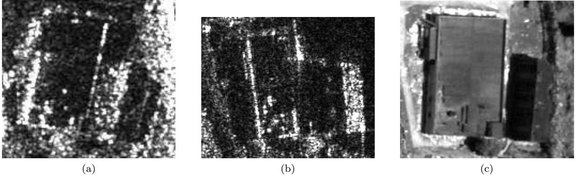
Figure 7.15: Interference of backscattering from buildings  $\omega_u^{[2]}$  and  $\omega_u^{[3]}$  ( $\omega_u^{[2]}$  is left from  $\omega_u^{[3]}$ ). (a) Subset of post-TSX scene with viewing direction from left. (b) Subset of post-CSK scene with viewing direction from right. (c) Subset of post-WV scene. (WorldView-1 image: DigitalGlobe distributed by Eurimage S.p.A, 2008; TerraSAR-X image: Infoterra GmbH/DLR, 2008; COSMO-SkyMed image: ASI distributed by eGeos S.p.A., 2008.)
