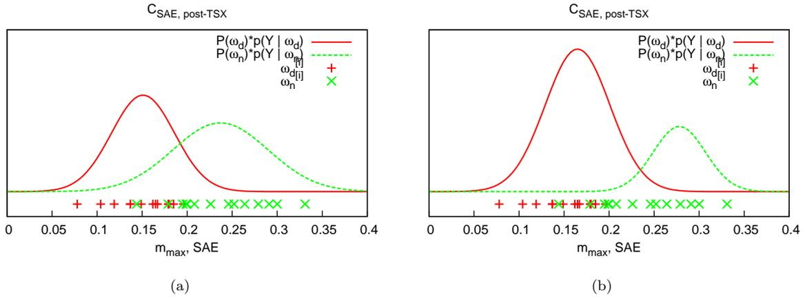
Figure 7.14: Comparison between supervised and unsupervised  $C_{SAE,post-TSX}$  classifiers. In this example the EM algorithm estimated the parameters for the unsupervised classifier inaccurately. The symbols “+” and “x” denote the actual  $m_{max}$  values of the buildings in class  $\omega_d$  and  $\omega_u$ , respectively. (a) Supervised classifier. (b) Unsupervised classifier.
