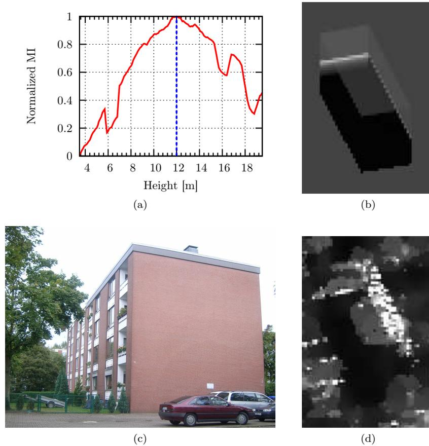
Figure 6.9: Results for building *A-2*. (a) Plot of the MI values normalized between 0 and 1, with a maximum at 12.0 m. (b) Simulation of the flat roof building model with height 12.0 m. (c) Photograph from the outside of the building. (d) Subset of airborne VHR SAR scene showing building *A-2*, which is coregistered to the simulation shown in (b). (SAR image: Intermap Technologies GmbH, 2003.)
