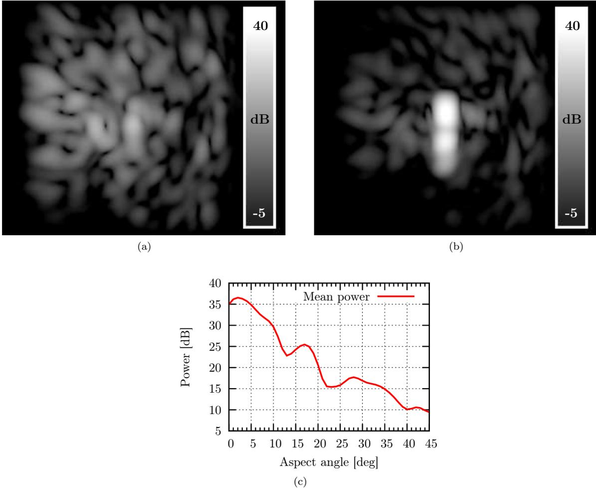
Figure 4.7: Example of the Pauli decomposition for the  $0^\circ$  aspect angle; (a)  $\alpha_p$ -channel; (b)  $\beta_p$ -channel; (black=-5 dB, white=40 dB). (c) Mean double bounce power (for the expected double bounce area) vs. aspect angle.
