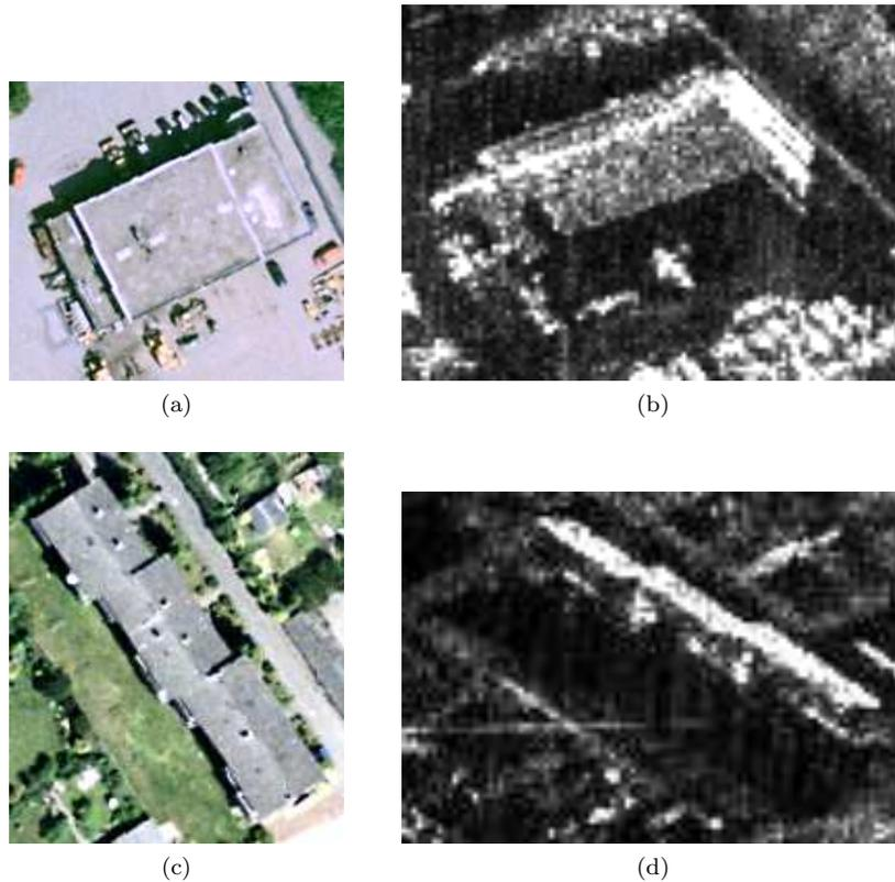
Figure 6.11: (a) Building *C-3* in orthophoto. (b) Building *C-3* in SAR image with viewing direction from the top. (c) Building *C-6* in orthophoto. (d) Building *C-6* in SAR image with viewing direction from the top. (Orthophoto: Landesvermessungsamt NRW, Bonn, 2007; SAR image: Intermap Technologies GmbH, 2003.)
