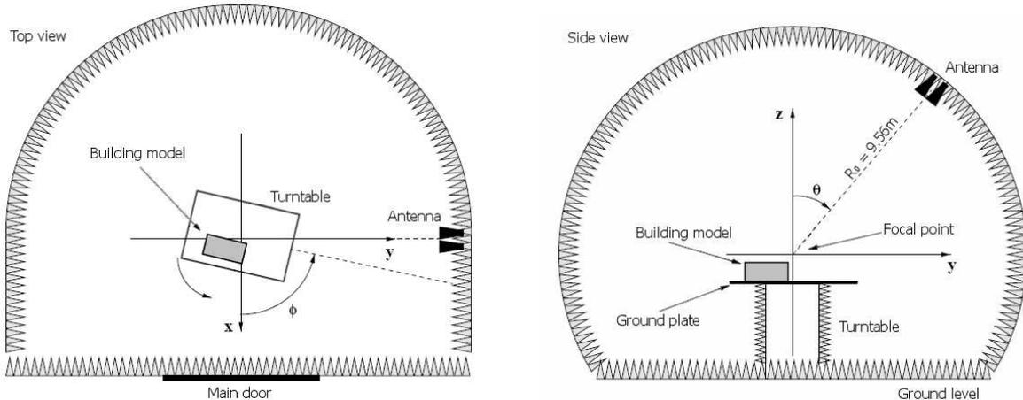
Figure 4.2: Schematic view of the EMSL and measurement setup of the experiment.
