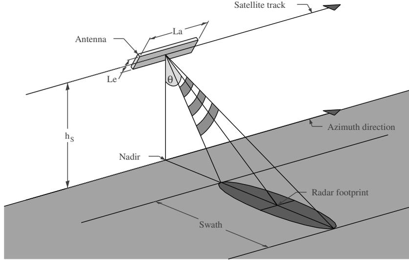
Figure 2.2: Side looking geometry of imaging radar systems.
