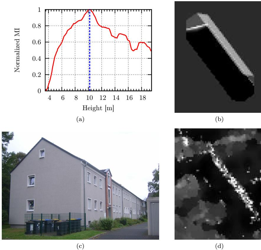
Figure 6.10: Results for building *B-18*. (a) Plot of the normalized MI values with a maximum at 10.2 m. (b) Simulation of the flat roof building model with height 10.2 m. (c) Photograph from the outside of the building. (d) Subset of airborne VHR SAR scene showing building *B-18*, which is coregistered to the simulation shown in (b). (SAR image: Intermap Technologies GmbH, 2003.)
