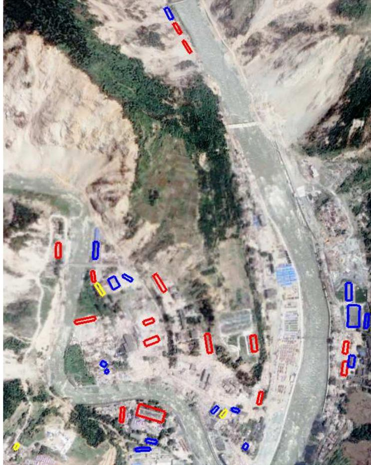
Figure 7.9: Footprints of selected buildings overlaid to the post-QB image, giving an overview of the distribution of the candidates in the test set. Buildings of class  $\omega_d$  are marked with red polygons, while blue polygons correspond to the class  $\omega_u$ . The yellow polygons show the three buildings where the true status in the post-TSX and post-CSK is unknown. (QuickBird image: DigitalGlobe distributed by Eurimage S.p.A, 2005.)
