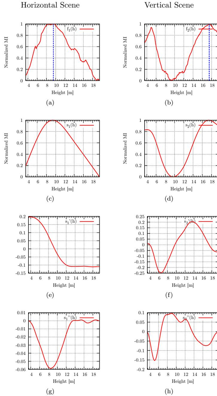
Figure 6.15: Intermediate results derived during the quality assessment and fusion procedure for building *A-3* in an interval from 3 m to 20 m. The left column shows the plots for the horizontal scene, while the plots in the right column refer to the vertical scene. (a) and (b) Original similarity functions. (c) and (d) Splines of the similarity functions. (e) and (f) First derivatives of the splines. (g) and (h) Second derivatives of the splines.
