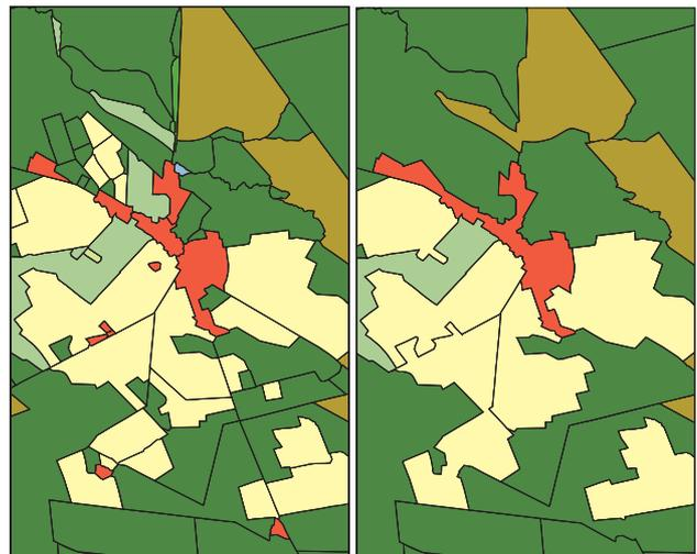
Figure 1: An example from the input data set at scale 1:50.000 (left) and a result for the scale 1:250.000 when minimizing changes of classes.
