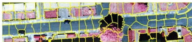
Figure 4. Segmentation without using road colour information derived from the database road.
