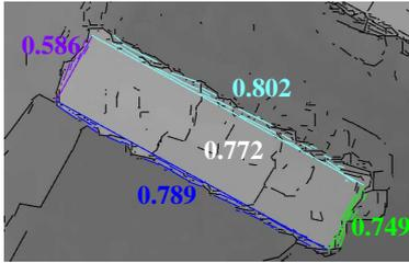
Figure 4: Description of the similarity measure. DSM contours extracted from the Canny-Derliche edge detector are pictured in black over the DSM. Each pertinent boundary is represented with its associated DSM contours and similarity measure. In white, the over-all similarity measure assigned to the building.
