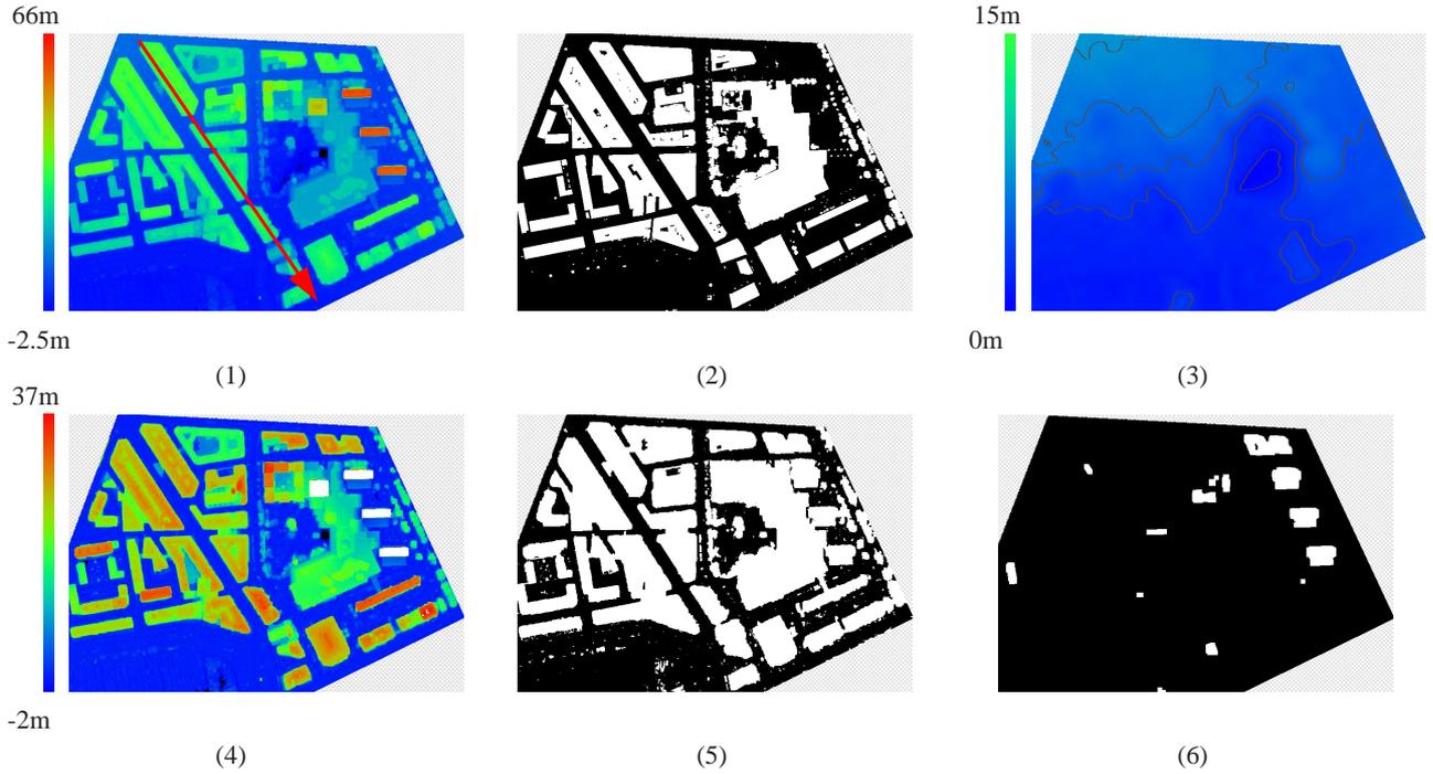
Figure 7: Detection of new buildings in Marseille. (1) : Initial DSM. (2) : Initial Above-ground Mask.  $\{Trees \cup Buildings\} - \{Destroyed Buildings\}$  (3) : Automatically processed DTM (Contour lines are superimposed over the DTM, with a contour interval of 3m). (4) : Building Height. (5) : Processed Above-Ground Mask. (6) : New building Mask.
