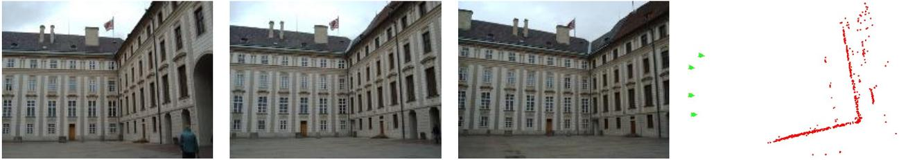
Figure 1: Three images of wide-baseline quadruple “Prague” and result after orientation and calibration (points in red, cameras as green pyramids;  $\sigma_0 = 0.24$  pixels)
