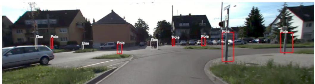
**Figure 4.** Projection of detected poles into the front camera image and classification based on the semantic segmentation image.
