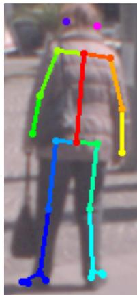
(c) Image section generated based on 3D bounding box, superimposed with the result of the image-based body pose estimation.
