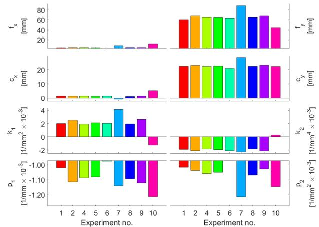
Figure 4. Deviations of interior orientation and distortion parameter values estimated by the proposed method from values estimated by reference calibration. Same scale for each left-right pair. Experiment 3 is not shown as some of its deviation values are by magnitudes larger compared to the other experiments.
