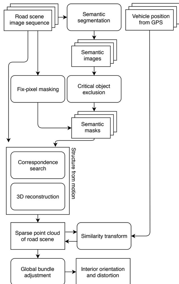
Figure 2. Workflow of the proposed method for robust self-calibration of a vehicle camera by using semantic road scene knowledge in a semantic-guided structure from motion algorithm.
