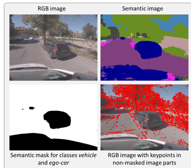
Figure 1. Top left: RGB road scene image as acquired by a vehicle camera. Top right: Semantic image obtained by semantic segmentation of the RGB image. Bottom left: Semantic mask obtained from semantic segments of the class *vehicle* and from the fix-pixel segment of the *ego-car*. Bottom right: SIFT feature keypoints detected in the RGB image considering only the non-masked image parts.
