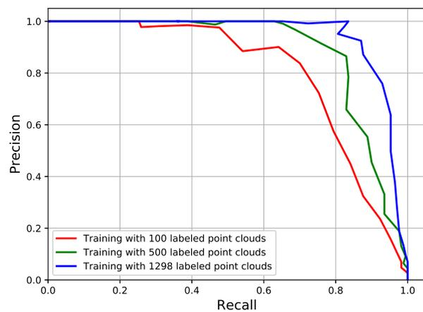
Figure 5. Results for different numbers of labeled point clouds used for training
