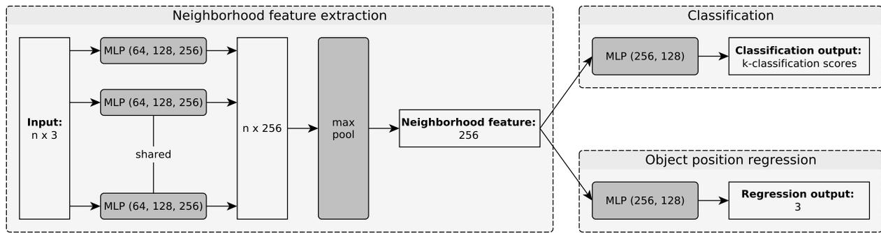
Figure 2. Chosen topology of the neural network. The network takes  $n$  3D points as input and it outputs a classification score for  $k$  classes and a 3D coordinate of the expected object center. MLP stands for *multi-layer perceptron*. Batchnorm is used for all the MLP layers, except the output ones. We use dropout layers with a dropout rate of 0.2 in the classification and regression part of the network but not in the feature extraction part.
