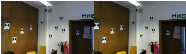
Figure 8. left and right image of a stereo pair of the ZED camera. Control points included. One can see that the corner of the room is left of the installation channel.
