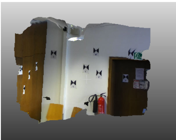
Figure 10. ZED Stereo camera point cloud colored with RGB intensities of the ZED camera.
