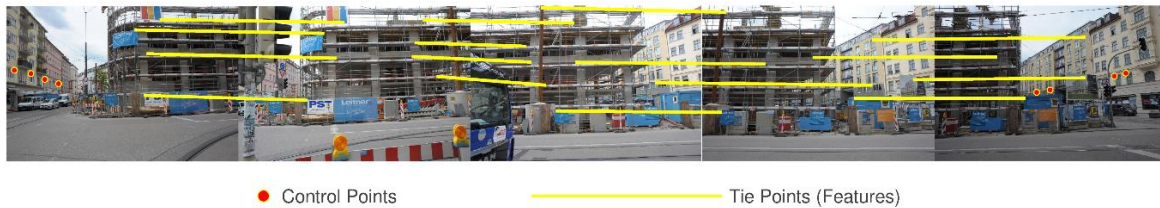
Figure 2: Image orientation process using control points and tie points
