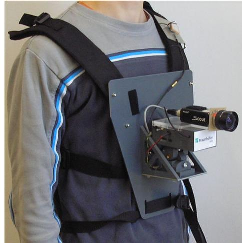
Fig. 1. Sensor system comprising an IMU and a camera attached to the torso of a person.
