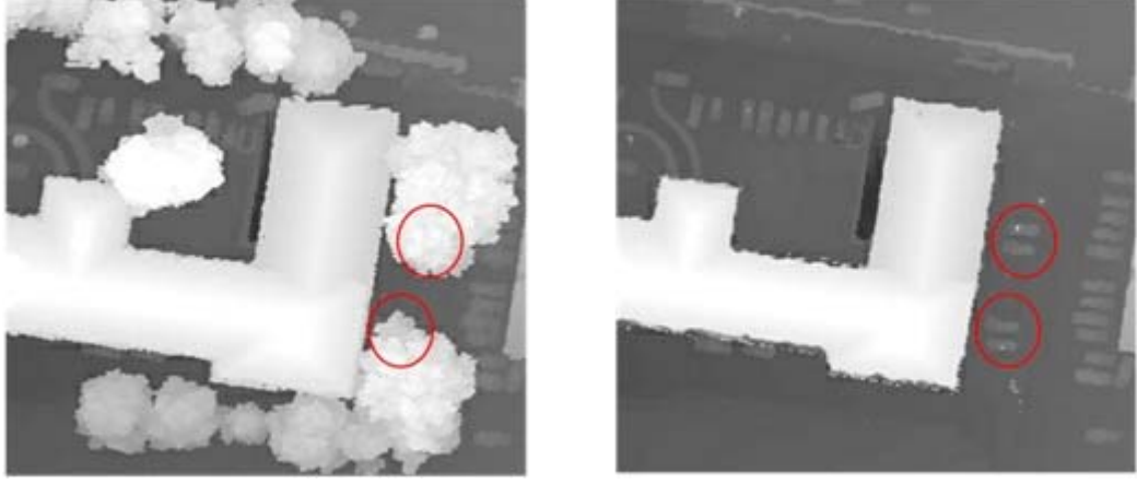
Figure 1: Airborne LiDAR range image illustrating the penetration ability of laser pulses through tree crowns to hit vehicles beneath, (a) first-pulse range image, (b) last-pulse range image (Stilla 2003)
