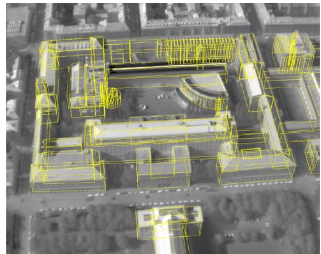
Figure 3. Projected model into a frame of a IR image using corrected INS/GPS data (Stilla et. al. 2009)
