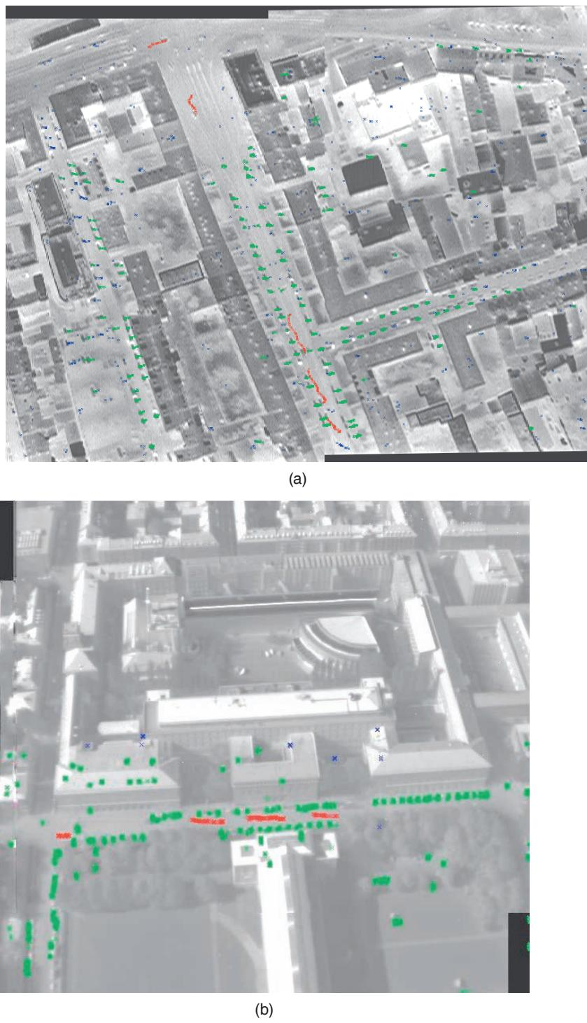
**Fig. 9:** Vehicle classification result in respect of movement: a) nadir view dataset, b) oblique-view dataset.
