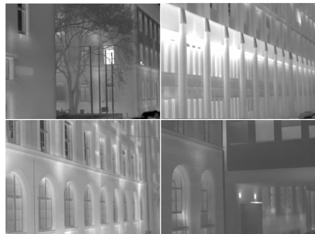
Fig. 2: a) several façades with occlusion, b) façade with regular structure, c) façade with irregular structure, d) façade with building bridge
