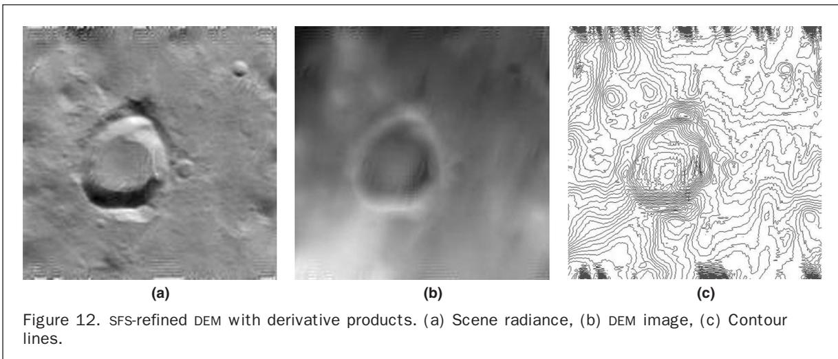
Figure 12. SFS-refined DEM with derivative products. (a) Scene radiance, (b) DEM image, (c) Contour lines.
