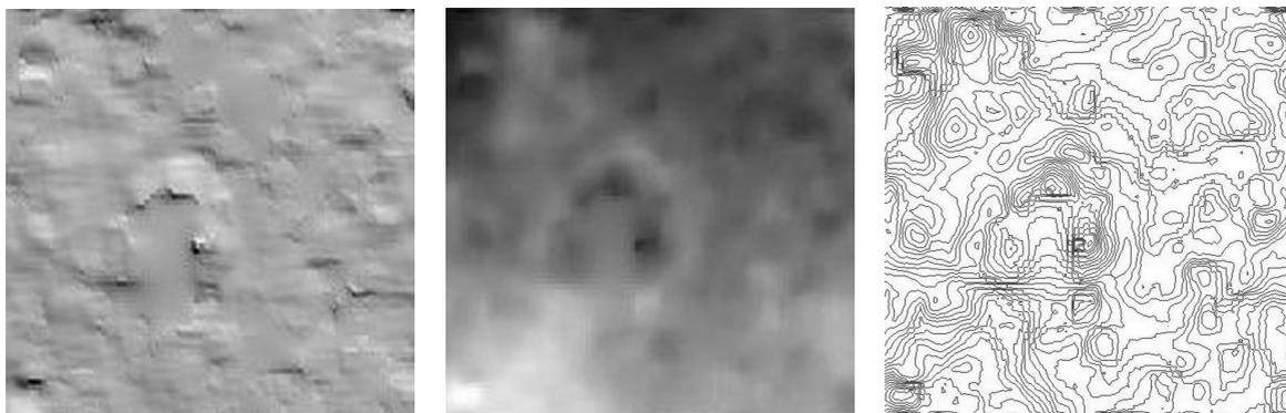
Figure 11. Initial DEM with derivative products prior to SFS. (a) Scene radiance, (b) DEM image, (c) Contour lines.
