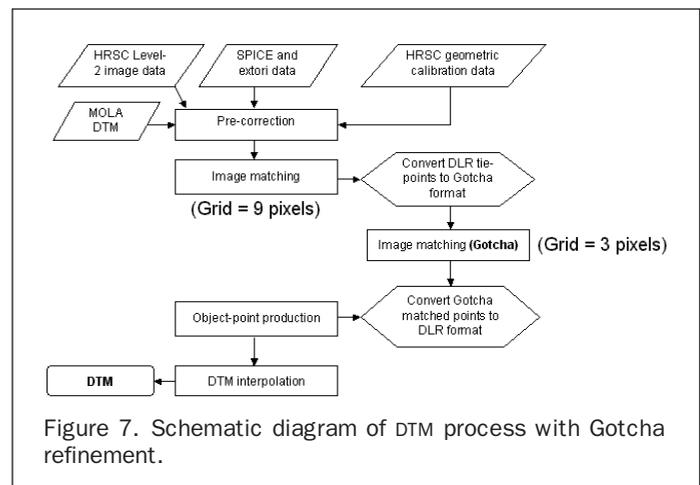
Figure 7. Schematic diagram of DTM process with Gotcha refinement.
