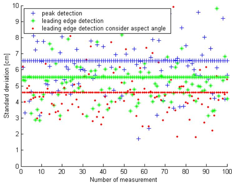
**Figure 9:** Standard deviation of the determined range for various detection algorithms
