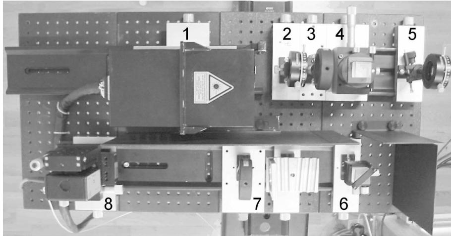
**Figure 2:** Experimental system. (1) laser, (2) half-wave plate, (3) double-concave lens, (4) beam splitter cube I, (5) quarter-wave plate, (6) beam splitter cube II, (7) double-convex lens, (8) receiver
