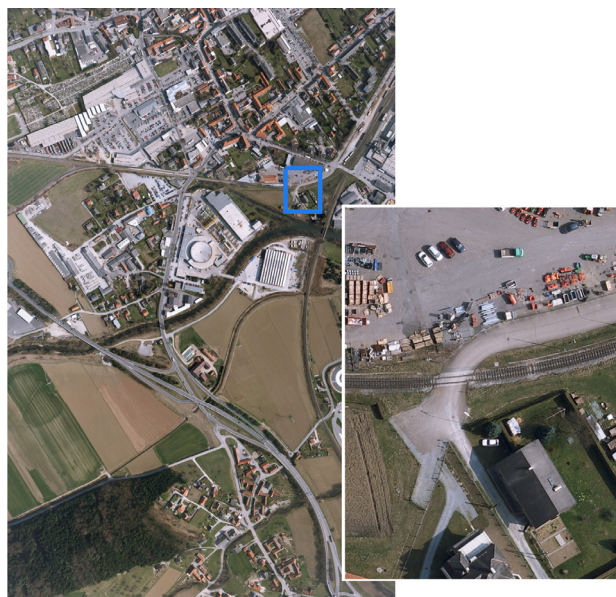
Fig. 3: Source image from UltraCamX at a format of 14430 by 9420 pixels. The entire frame is shown on the left, the detail on the right covers a footprint of 68 by 90 meter.
