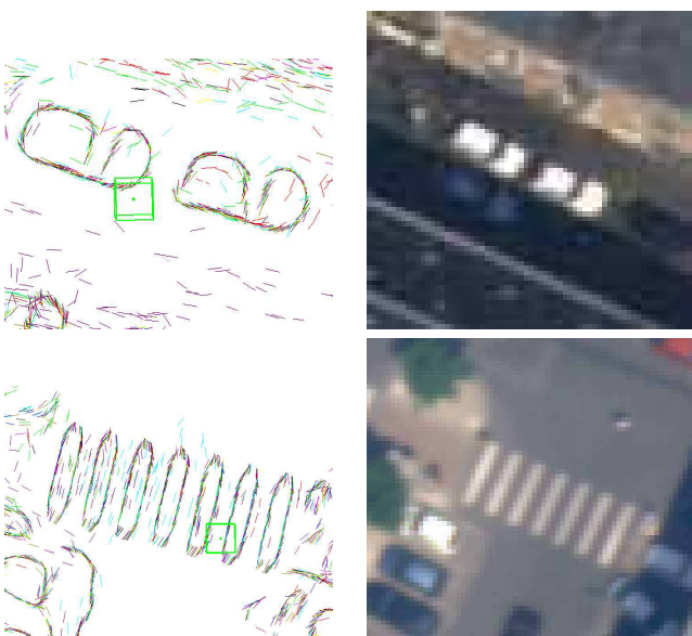
Figure 8: Example of non-linear object extraction with edgels. The shape of small objects (cars, zebra crossing, etc.) are well reconstructed using edgels. The square (upper left and bottom left images) is used as a 1m x 1m metric reference.
