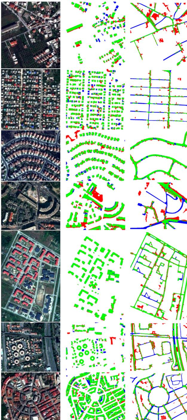
Figure 5. (first column) Test dataset (#1-7, RGB), (second column) the results of building regions, and (third column) the results of road regions. Green, red and blue colours represent true-positive, false-positive and false-negative, respectively.
