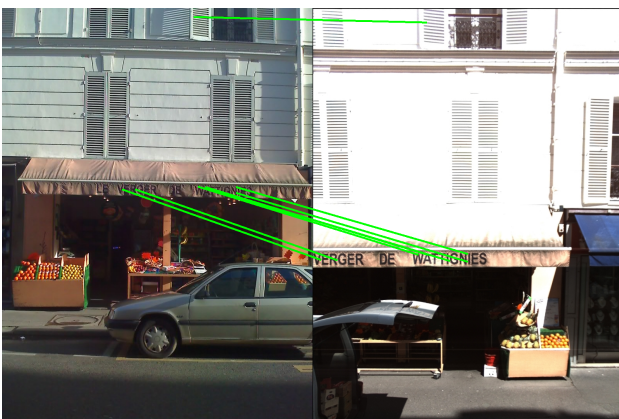
Figure 4: Matching points after the non-coherent to the estimate 2D affine transform matches have been remove.
