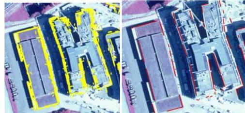
Figure 9. Left: the straight lines which may belong to the building outline (yellow) and Right: long lines (red).
