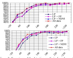
Figure 9. Correctness of the detection results in dependence of the building size [m²] for the four variants described in the text [%]. Above: Fairfield, below: Memmingen.
