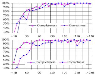
Figure 8. Completeness and correctness of the detection results as a function of the building size [m²] for Fairfield (above) and Memmingen (below).
